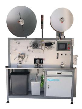
5. Cutting system: equip with Guidance mechanism and precision cutting wheel, cut off redundant tapes ,the carrier tape will be with right width size.offcut tapes will automatic running out.
