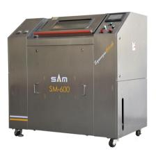
SMT Squeegee Cleaning UNIQUE FEATURES Innovative design , rotation ultrasonic combination with spray clean Equip with pneumatic pump , auto add and drain clean solvent Inching holder , easy load unload squeegee Install with solder paste reclaim bags Stainless steel chamber and filter , Durable and corrosion resistance Easy setting & operation Easy maintenance CONTROL SYSTEM PLC Control touchsceen
